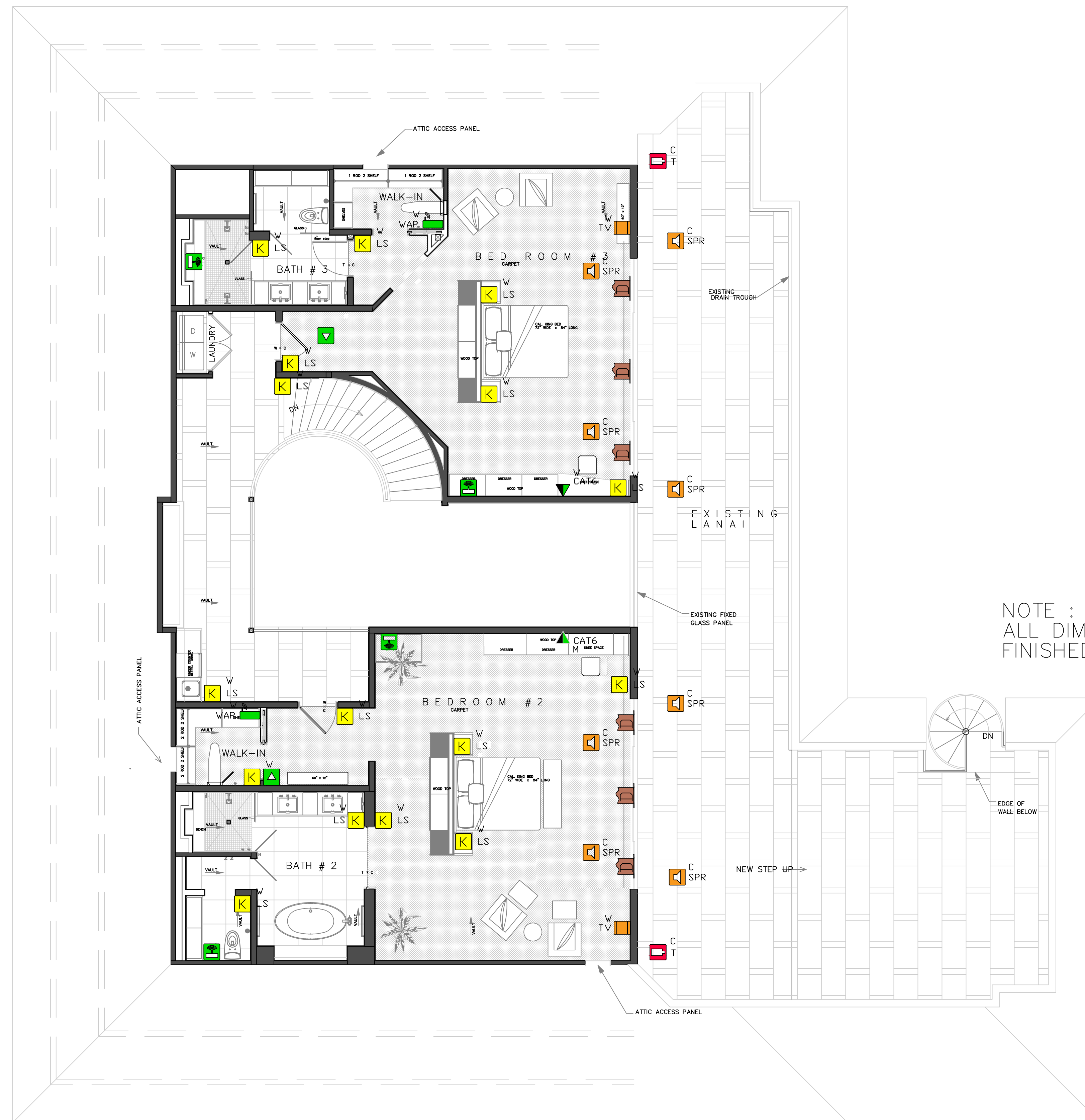
3 UPPER LEVEL DEVICE LOCATION EXHIBIT SCALE : 1/4" = 1'-0"
